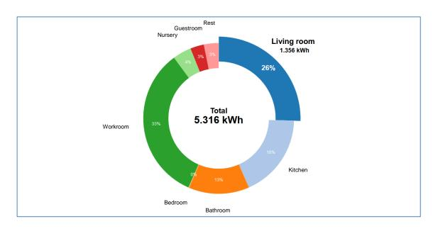
Figure 2.5 Day view pie graph, percentage distribution per power circuit
