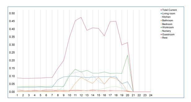
Figure 2.4 Day view line graph in kWh per power circuit and hour
